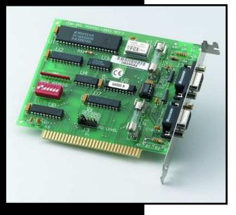
Keithley's COM-485 board allows ISA-bus compatible computers to be networked over the RS-485 bus. Unlike the RS-422 bus, which allows multiple receivers but only a single transmitter, the RS-485 allows multiple transmitters and receivers to communicate over a 2-wire bus allowing a "party-line" network configuration. The COM-485 allows up to 32 different driver/receiver stations to communicate at 115.2 kbaud. COM-485 stations can be located up to 4000 feet away from each other.
